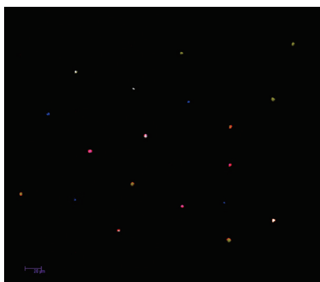
Figure 5. Confocal fluorescence image of a mixture of eight types of MNSs-IBU under 488 nm argon-ion laser excitation.
